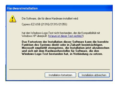
This process must be repeated twice, as two different drivers (Cypress EZ-USB and RFID Reader) must be installed.
